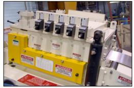
them to the stamped material. We also ordered the straightener with hard-chrome and polished rolls, because these give the least amount of pickup," added McLaren. So the company performs a daily cleaning (wiping down the rollers with a simple alcohol solution) and does so quickly...simply opening it up by loosening two screws, completing the entire operation/cleaning process in a matter of minutes.
