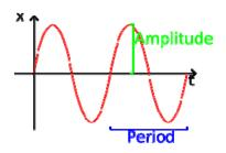
The displacement, x, as a function of time. The amount of time that passes between peaks is called the period. The mass of the spring is assumed small in comparison to the mass of the attached mass and is ignored. Since acceleration is just the second time derivative of x,
