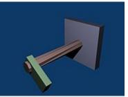
A torsion bar twisted under load
