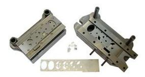
**Progressive stamping** is a metalworking method that can encompass punching, coining, bending and several other ways of modifying metal raw material, combined with an automatic feeding system.
